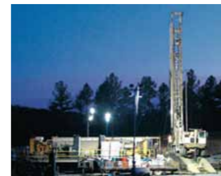
The RD20 is a high production rig with capability to drill wells to depths in excess of 5,000 ft.
