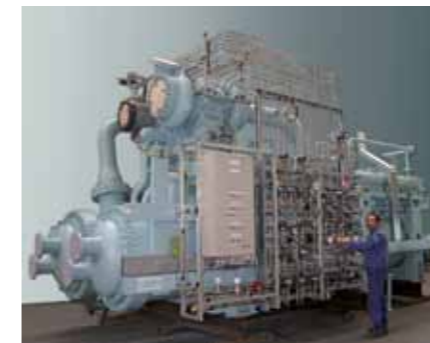
A Comander for on-board reliquefaction of LNG.
